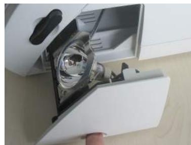
First of all switch off the light source and pull out the mains plug.
