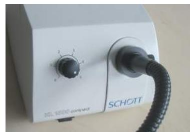
First undo the fixing screw (3) of the light guide socket (2) by turning in an anti-clockwise direction. Push the light guide in as far as the stop and tighten the fixing screw by turning clockwise.
